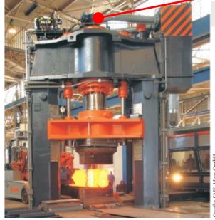
Push-down type forging press with two columns
