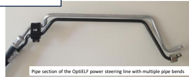
Pipe section of the OptiELF power steering line with multiple pipe bends
