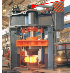
Push-down type forging press with two columns
