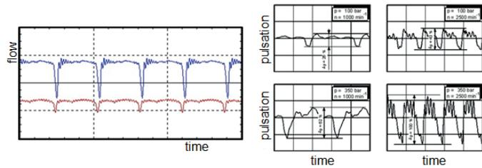
Figure 5: real pump flow /7/ and measured decompression effects /9/
