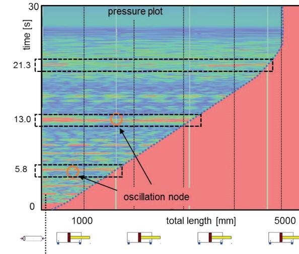
Figure 18: 2D pressure plot for model B
