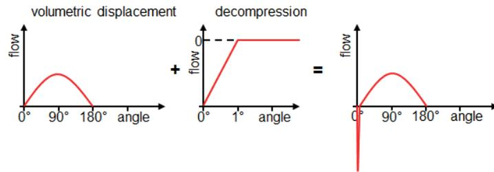
Figure 3: pump flow parts of one cylinder
