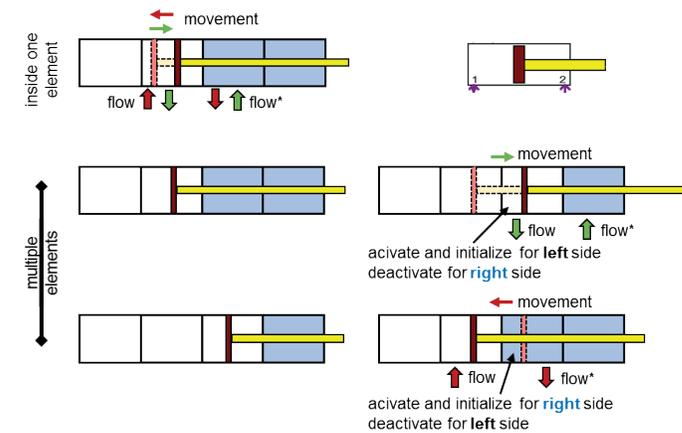
Figure 15: distributed cylinder with deactivated intermediate element
