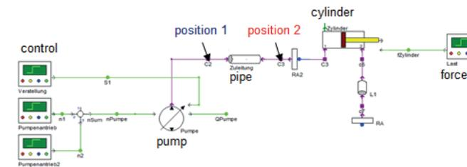
Figure 16: model B with distributed parameter pipe and cylinder
