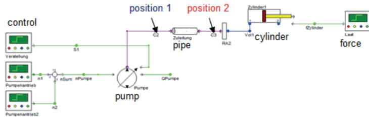
Figure 8: model A with distributed parameter pipe and classical cylinder
