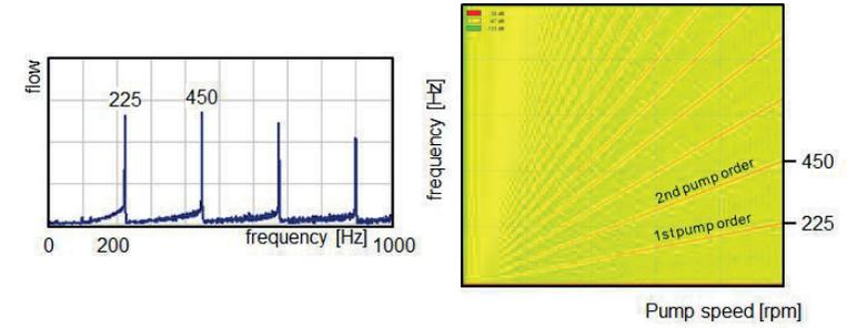
Figure 6: frequencies of pump flow at 1500 rpm an Campbell-diagram of a pump run-up
