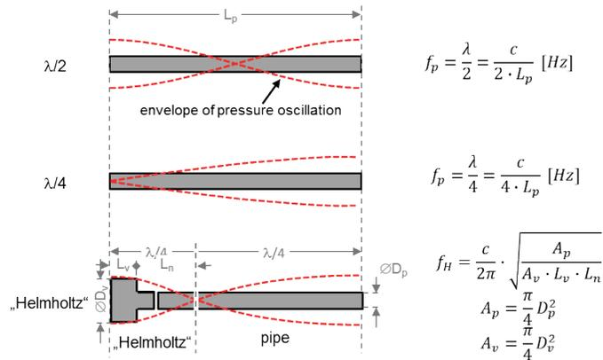
Figure 10: first oscillation modes and “Helmholtz” like frequency
