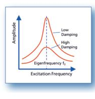
Whether hitting a resonance will result in problematic pressure pulsations or not depends on the systems damping characteristic, the initial pressure amplitude of the excitation and the position of the excitation source within the system. RohrLEx illustrates the formation of a resonance as follows.
