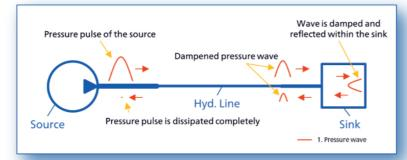
Due to internal friction within the fluid, partial reflection at fittings or diameter variations and especially due to the visco-elastic properties of hose walls (if present) the pressure amplitude is constantly reduced while running through the system. As a result a part of the pressure wave's energy is dissipated into heat, the remaining pressure pulse reaches the last element connected to the line and might experience further damping.
