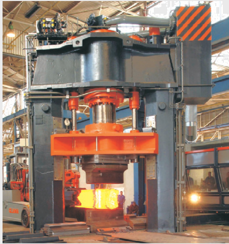
Push-down type forging press with two columns
